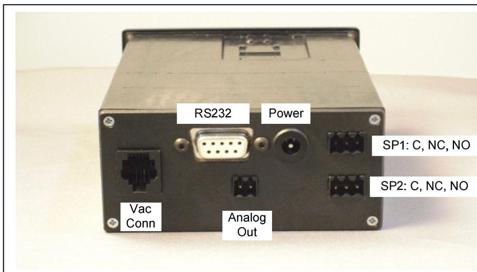
2. **N.C.** - Normally closed. This means that above the set point value there is a current path between the common and the N.C. terminal. Put another way the switch is "ON" between these 2 terminals. At the set point value and below (higher vacuum, lower pressure) the connection is open. Put another way, the switch is "OFF" between the common and the N.C. connection at higher vacuum (a lower vacuum reading).
