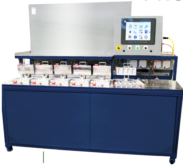
Multi-chamber helium leak test system for medical diagnostic devices.
