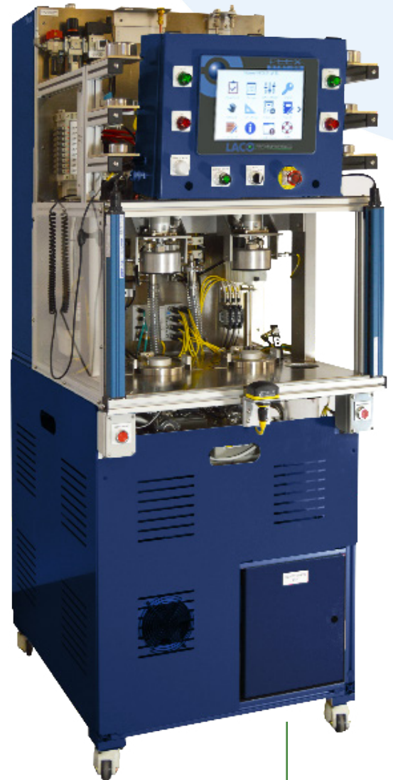
Dual chamber helium leak testing system for airbag inflators with 3 second cycle time, and leak testing to 1 \times 10^{-5} atm.cc/sec.
