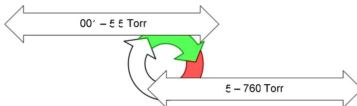
Similarly as the pressure level is decreased from 760 Torr to 5 Torr, the vacuum reading is taken from the transducer. At 5 Torr, the vacuum reading transitions to being taken from the Thermocouple.
