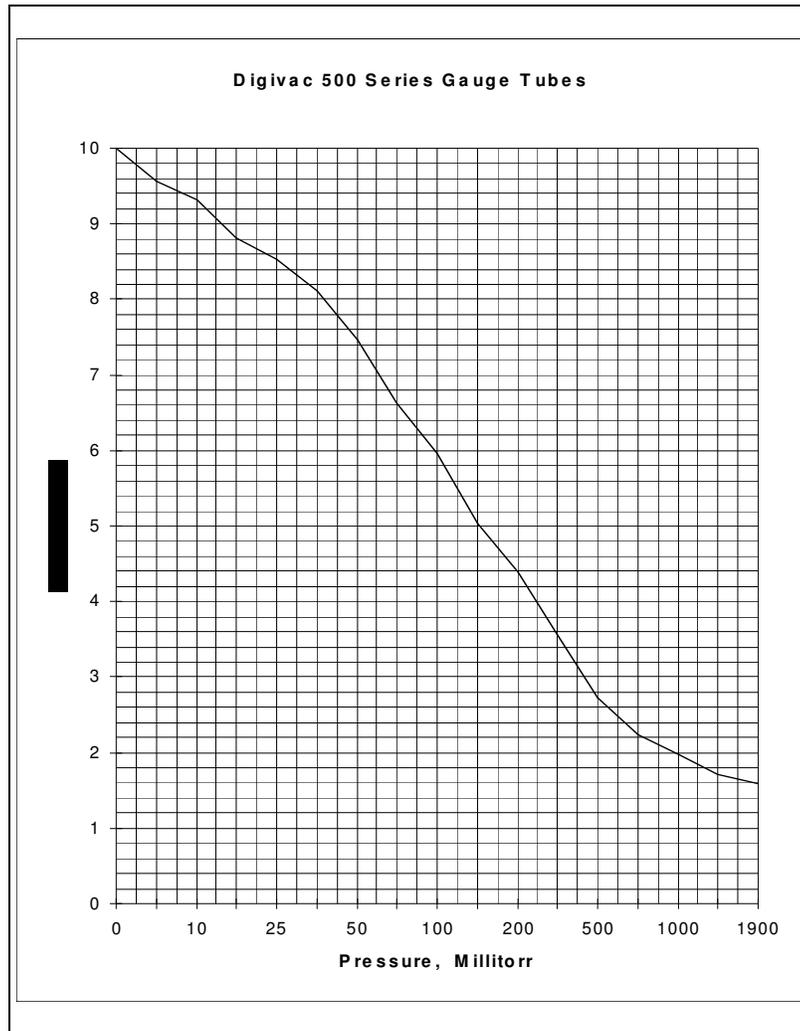
Typical response of a Hastings Dv-6 and Dv-36 tubes
