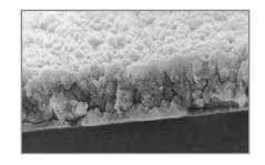
$Al_2O_3$  sputtered with the aid of an  $AE^{\oplus}$  pulsed-DC product (left)
