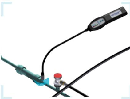
Screwed unions or other connection points must be „scanned“ slowly, i.e. move the sensor head (3) right around the complete connection point.
