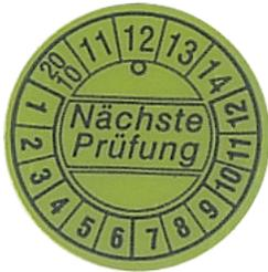
It is necessary to arrange for annual inspections by the manufacturer, a service company or instructed staff. The inspection sticker adhered to the device housing shows when the last inspection was carried out and indicates the date of the next one.
