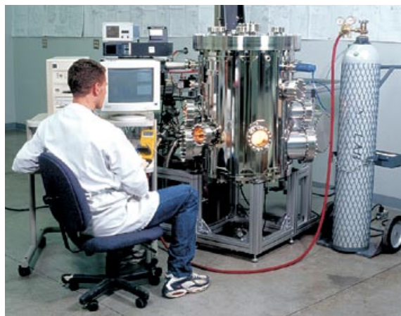
Leak testing of chamber on chamber qualification test bench
