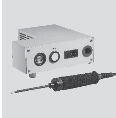
Helium sniffer QUICK-TEST QT 100 with sniffer
