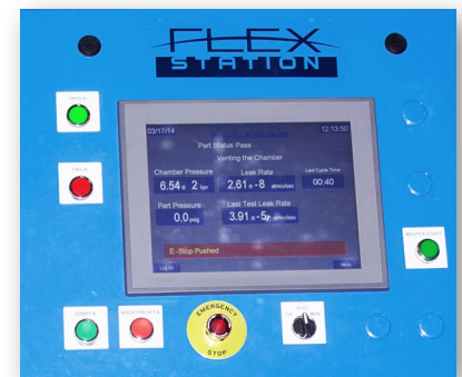
Industrial PLC with 10" color touch screen
