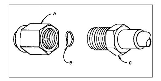
*Figure 8-1: Parker CPI UltraSeal coupling—O-ring removal tool usage (standard fitting)*
