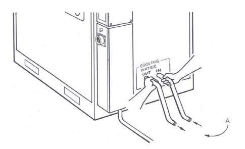
Figure 3-27: Cooling water flow direction check
