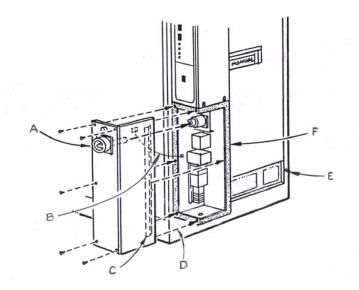
Figure 3-10: High Voltage Box Panel Removal; External Ground Stud Locations
