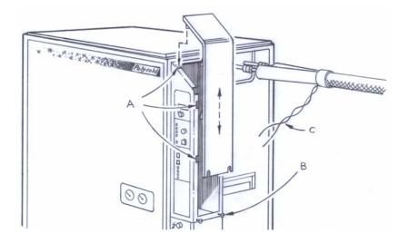
Figure 3-22: Low Voltage Box Panel Removal
