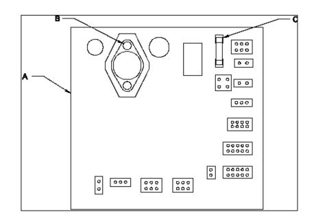
*Figure 3-9: Control Voltage Check—Voltmeter Connections*
