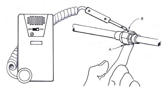
Figure 3-19: Couplings—Leak-checking Method
