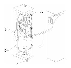
Figure 3-11: High Voltage Box Component Locations
