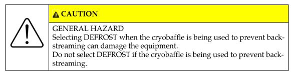
**NOTE:** Backstreaming will contaminate the system because it is the process of hot vapor migrating and condensing on cold surfaces. When the vacuum pump is used, the pump oil heats up and travels opposite of the pumping direction and condenses the system resulting in system contamination.
