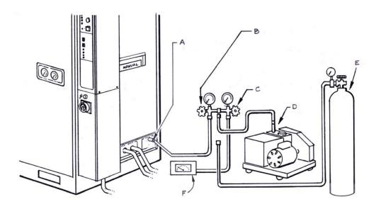
*Figure 3-20: Refrigerant Line & Cryosurface – Evacuation Set-up*
