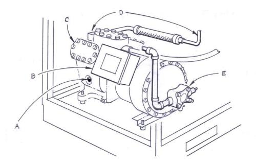
Figure 3-26: Compressor parts location
