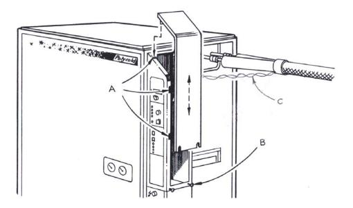
Figure 3-30: Low Voltage Box Panel Removal
