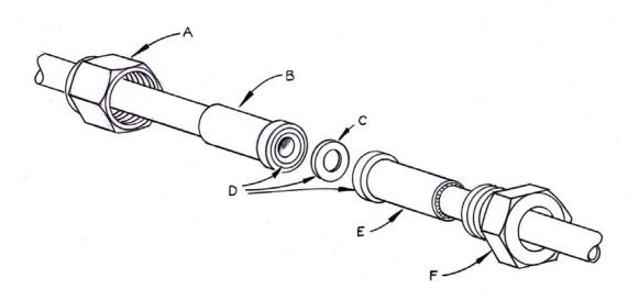
Figure 3-14: Cajon VCR Coupling (optional fitting)
