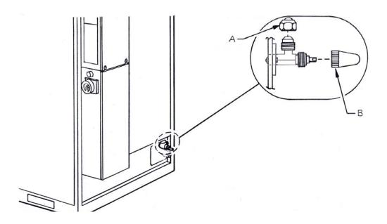
Figure 3-21: Evacuation Valve Closure
