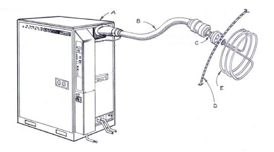
*Figure 1-1: PFC cryopump – primary application*
