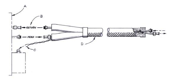
Figure 3-15: Refrigerant line connection
