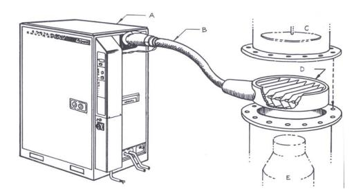
*Figure 1-2: PFC cryopump*—secondary application
