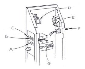
*Figure* 9-10: *Temperature module options*—*parts identification for option* 600212-03
