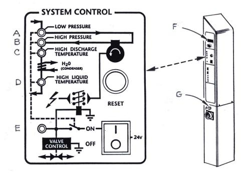
*Figure 7-1: Unit indicator lamps*
