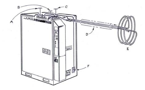
Figure 3-17: Evacuation Valve, Refrigerant Line & Cryosurface Relationship
