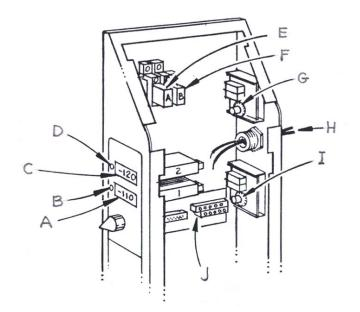
*Figure* 9-11: *Temperature module options*—parts identification for option 600212-04
