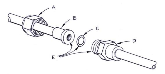
Figure 3-13: Parker CPI UltraSeal coupling (standard fitting)
