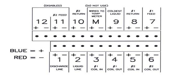
Figure 3-23: Thermocouple (TC) positions identification
