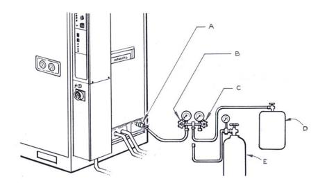
*Figure 3-18: Refrigerant Line & Cryosurface – Leak-check Charging Set-up*
