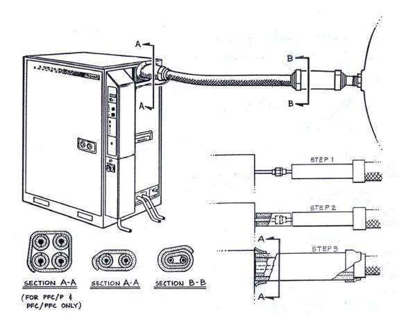
Figure 3-25: Insulating Exposed Tubes and Couplings Method
