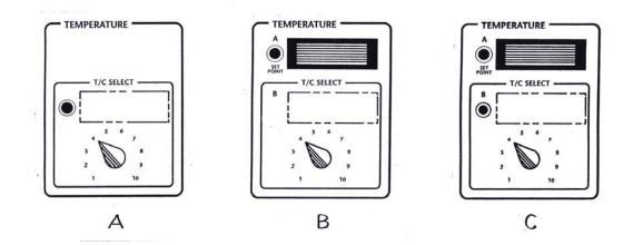
Figure 9-8: Temperature module options identification
