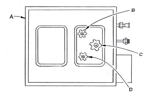
Figure 3-16: Isolation Valves Location
