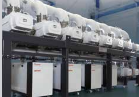
Application example customized system solution: Steel degassing applications comprising 4x DRYVAC DV 1200 and 10x RUVAC WH roots blowers Max pumping speed: 59,000 m 3 /h (34,760 cfm)
