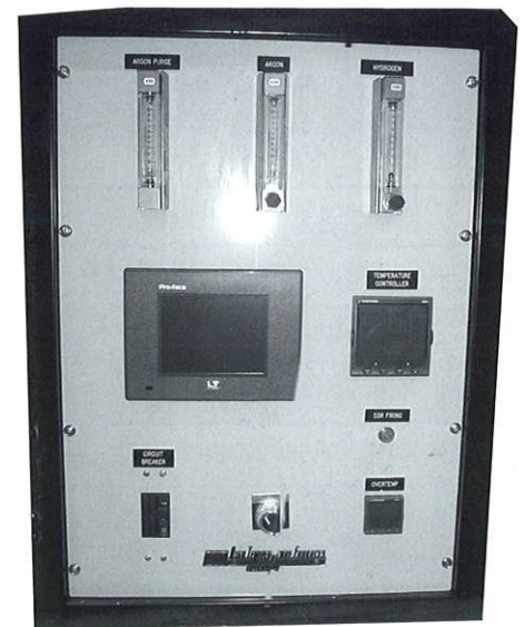
1200 with retort and hydrogen atmosphere option
